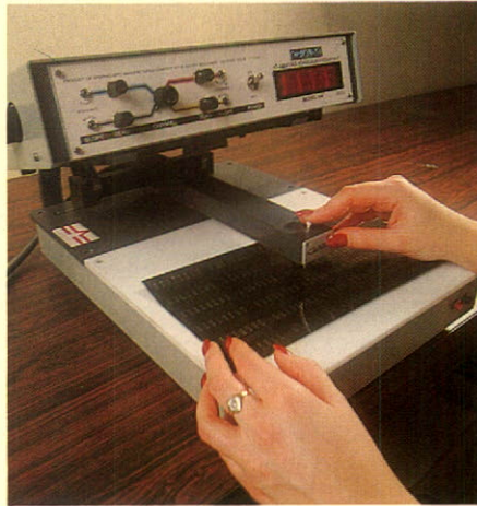
The densitometer is one device to ensure printing quality at Neeco Industries.
