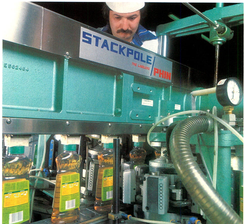
A Canadian made labeller, part of Chempac's high speed liquid filling line.
