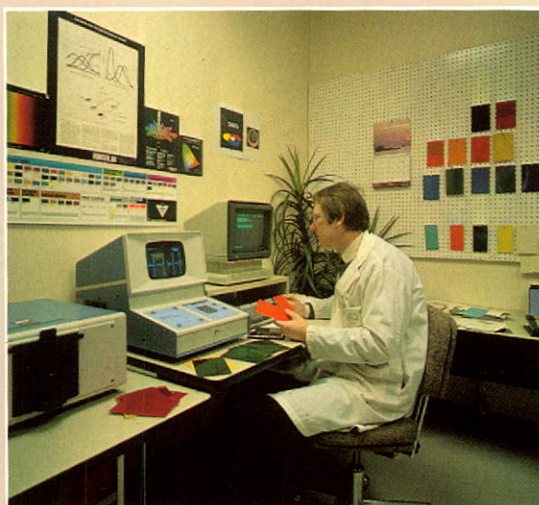
▲ Colour matching and batch corrections are simplified by the use of a scanning spectrophotometer and digital computer.
