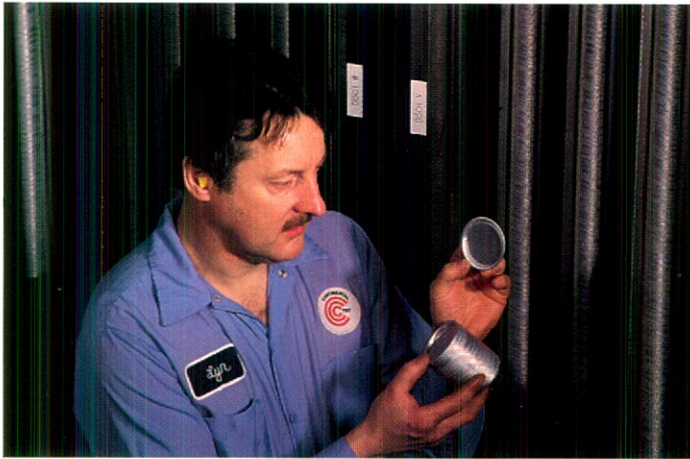
Lyn Webb - Maintenance Technician Reviewing quality of aluminum end units produced on a 10-out Shell Press.
