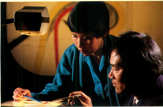
Joy Young - Research Engineer Hwa Shik Shim - Research Engineer Quality control inspection of a double side seam via overhead projector.
