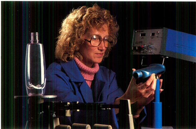
Dallis Holmes - Quality Control Supervisor Determining material distribution in plastic containers using digital read-out Magna Ball system.
