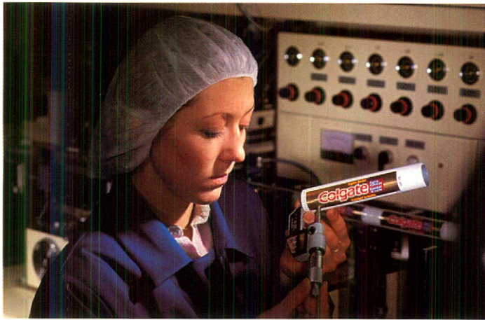
Susan Baker - Quality Assurance Inspector Measuring the wall thickness of a laminate tube to ensure it meets specifications.
