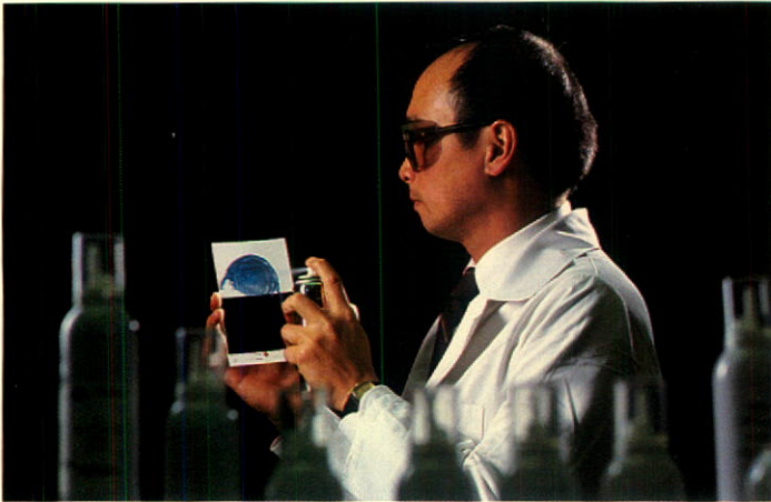
Recto Yee - Manager of Technical Services Verifying that the spray characteristics and colour match for a hair spray product meet specifications.
