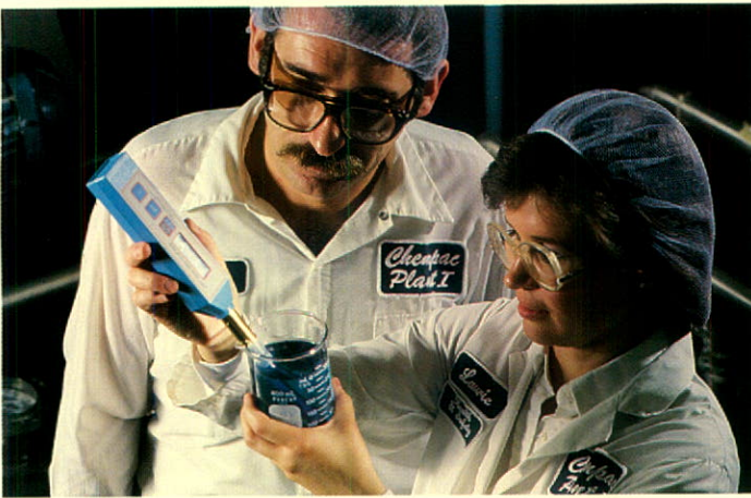
Kris Kordis - Compounding Supervisor Laurie Cressman - Laboratory Manager Checking the pH of a shampoo batch before final release is given to fill the product into bottles.
