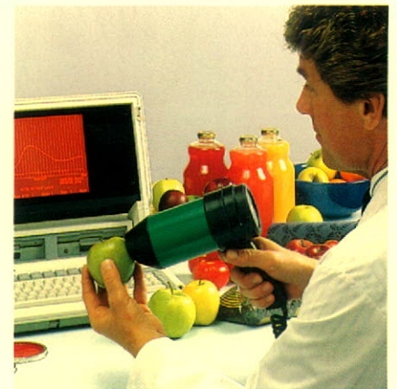
One of the Company's newest technologies, the Colormet spectrophotometer is used to test colour in plastics, paints, foods and various other substances.
