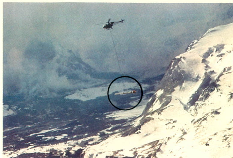
The Dighem System shown surveying Mount St. Helens. The United States Geological Survey employed Dighem to detect geothermal activity in the volcano. The "Bird" towed beneath the helicopter contains electromagnetic transmitting and receiving coils. Photo courtesy of U.S.G.S.
