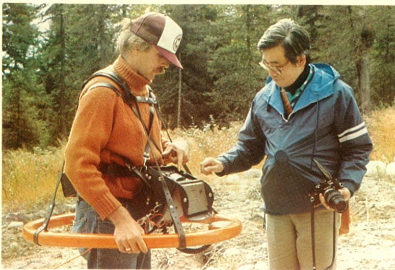
Ken Thorsen of Teck Explorations and N. Ogushi of Dowa Mining using an electromagnetic survey instrument to locate hidden ore deposits.
