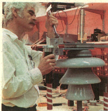
Detection device for locating faulty insulators.
