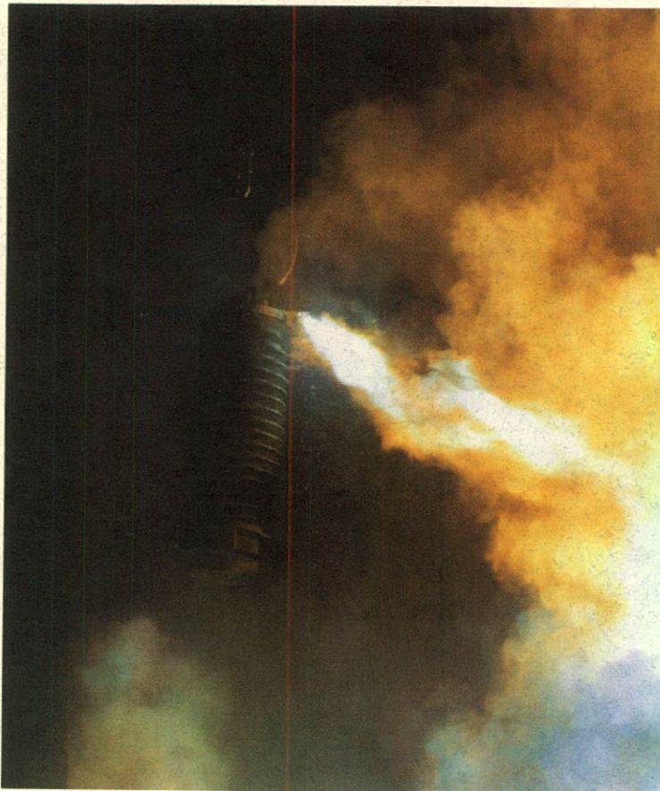
Internal arcing during tests on distribution surge arresters at the high-power laboratory.
