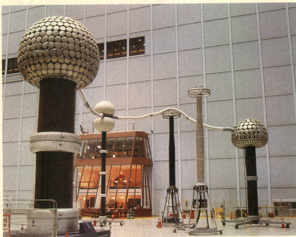
Tests on 500-kV DC cables in the main ball of the high-voltage laboratory.
