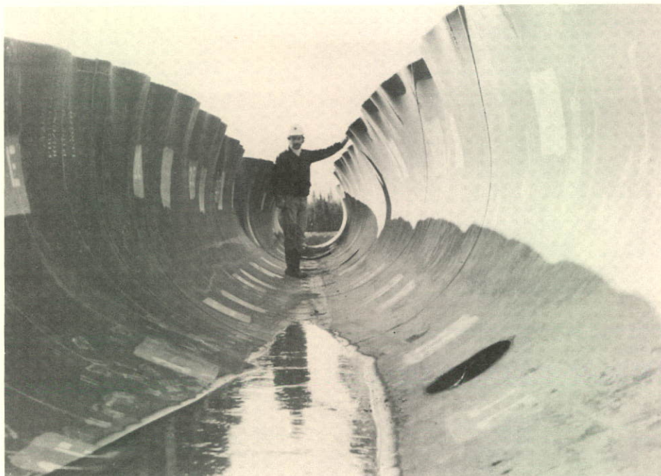
A section of pipe torn apart at the burst-test facility, Rainbow Lake, Alberta.
