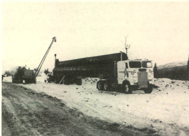
On a successful test drive from Edmonton, a specially designed tractor-trailer unit, which is capable of tracking automatically from the rear, arrives at the Quill Creek test facility in Yukon. The trip was made to test the new vehicle's ability to carry long joints of pipe around sharp corners such as those along the Alaska Highway.
