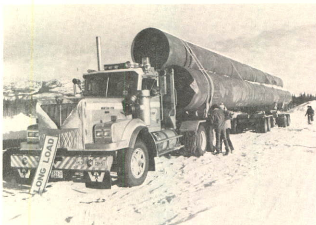
Self-Steering rear assembly of a four-axle tractor-trailer loaded with 23-m (76-ft.) lengths of pipe for test runs along the Alaska Highway.
