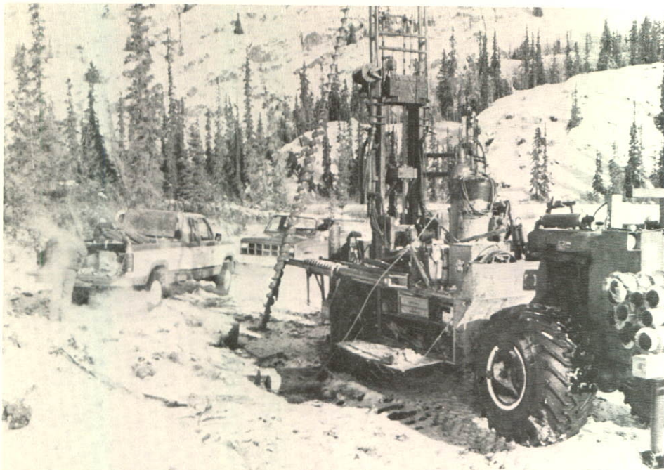
Geotechnical crew sets up drill to take core sample along the Alaska Highway near Marsh Lake in Yukon.
