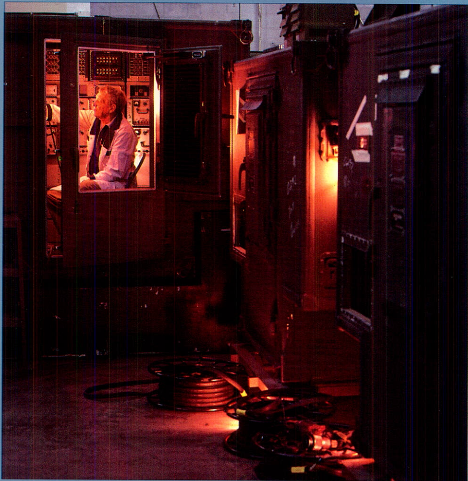
U.S. Army shelter-mounted communications systems are upgraded to become CMC's AN/TRC-180. The radio terminal system, mounted on the back of a truck, provides a central relay point for communications in the field.
