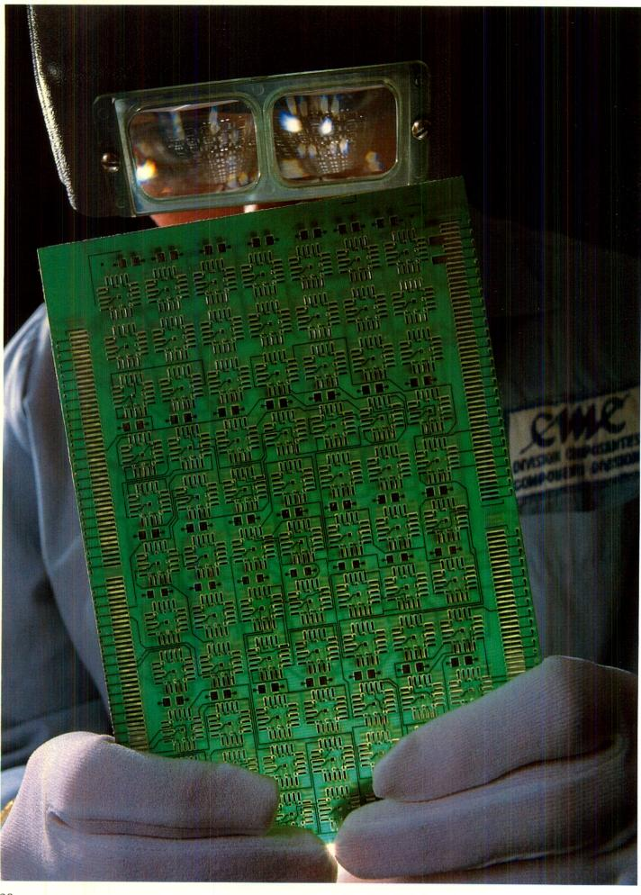
A Leadless Chip Carrier (L.C.C.) printed circuit board at one of many inspection stages.
