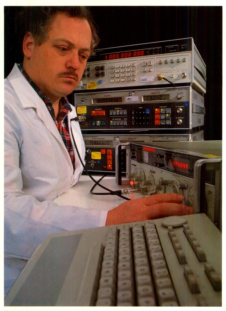
The Special Services Division's Electrical Standards Lab is dedicated to the support of both electrical and mechanical test apparatus. The photograph shows a senior metrologist using sophisticated, automated equipment in conjunction with a computer to calibrate a signal generator.
