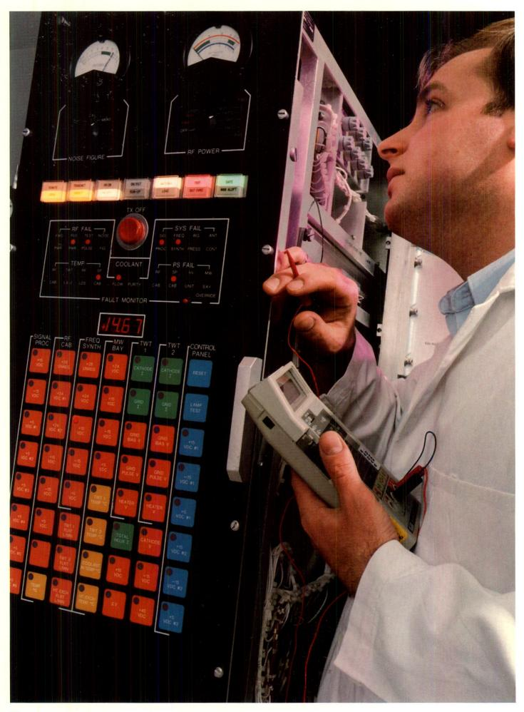
The AN/SPS-503 is a prime example of CMC's innovative radar technology. Originally developed for the Canadian Navy's Destroyer Life Extension (DELEX) Program, this medium-range shipboard surveillance system incorporates enhanced features of flexible design. In the photo, a fully assembled receiver transmitter bay is undergoing a voltage check.
