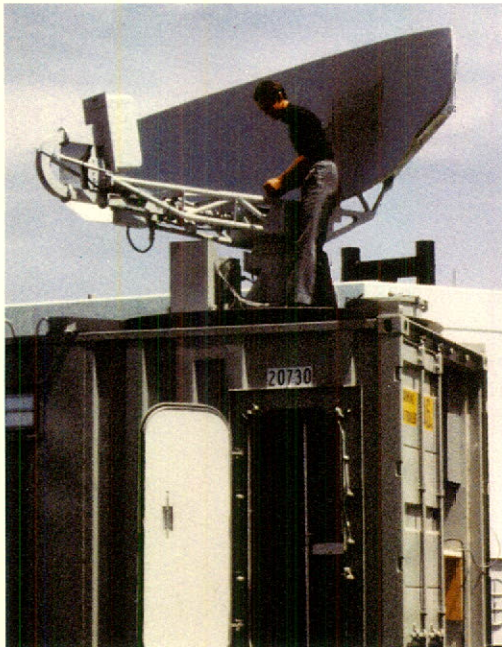
Test installation of the AN/SPS-503 naval surveillance radar antenna for Canada's DELEX Program. The transmitter-receiver assembly is housed in the container below. Photo: courtesy Mark Edwards
