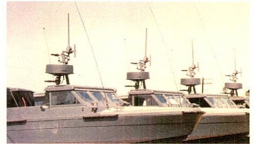
The U.S. Navy's SEAFOX craft use the LN-66 radar for short range surface search and navigation purposes. Photo: courtesy D. Davies
