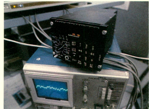
A prototype GPS receiver undergoing engineering tests.
