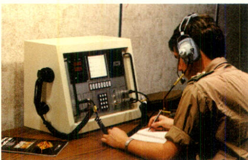
Canadian Marconi's new Operator's Console developed as part of an Air Defence System for a country in the Middle East.
