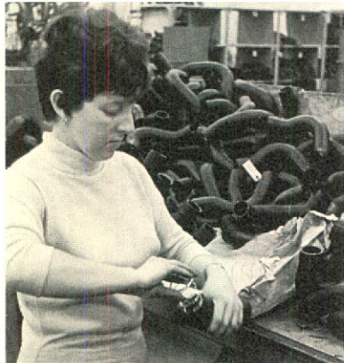
Employee inserts stiffener spring in automotive hose and inspects it.
