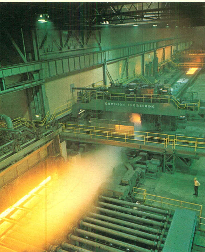
Slabs for the plate mill are discharged from the unique "walking beam" reheat furnace. They are then reduced by the 2-hi roughing stand and moved downstream to the 4-hi finishing stand.
