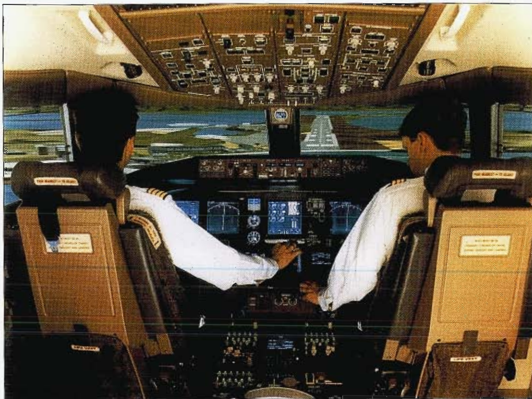
CAE 777 flight simulator; the first in the world for the Boeing Commercial Airplane Group
