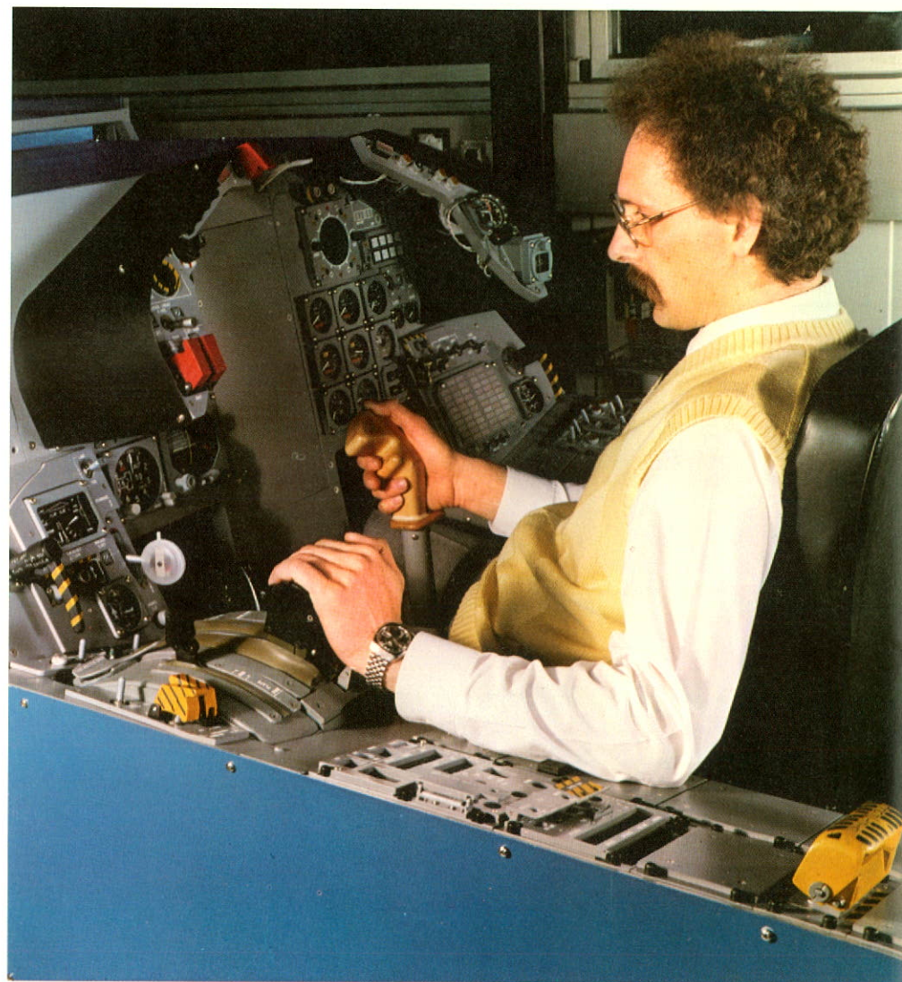
MRCA Tornado engine trainer by CAE Electronics GmbH for German Armed Forces.
