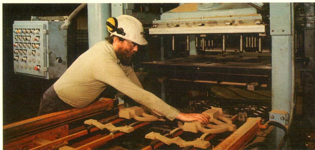
Engine manifold cores being prepared at CAE-Montupet DieCast Ltd.
