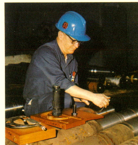
Checking close tolerance machining of railway axle journals at Canadian Bronze Company Limited.
