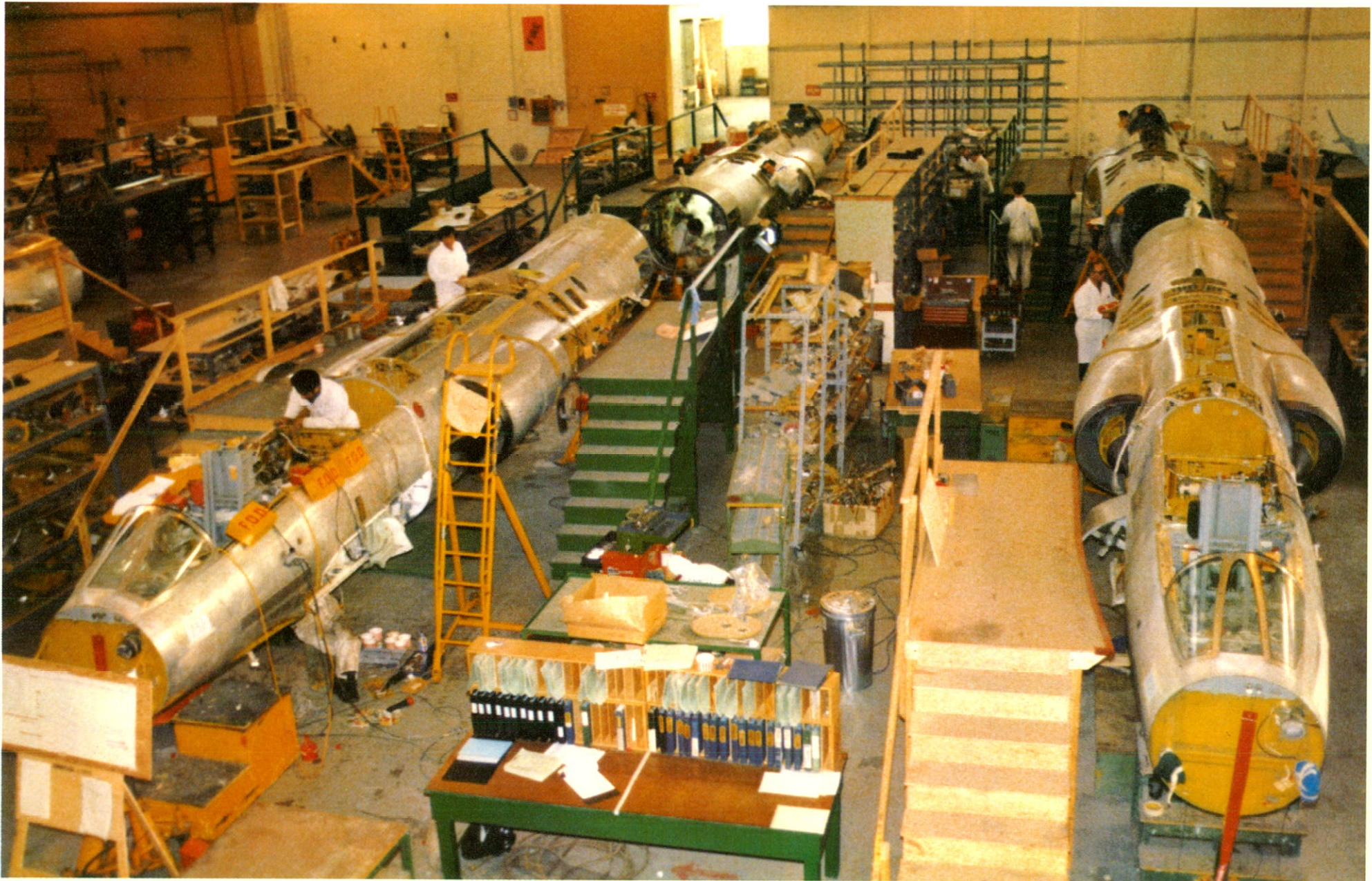
CF-104 Starfighter aircraft of the Canadian Armed Forces undergoing major maintenance at Northwest Industries Limited.
