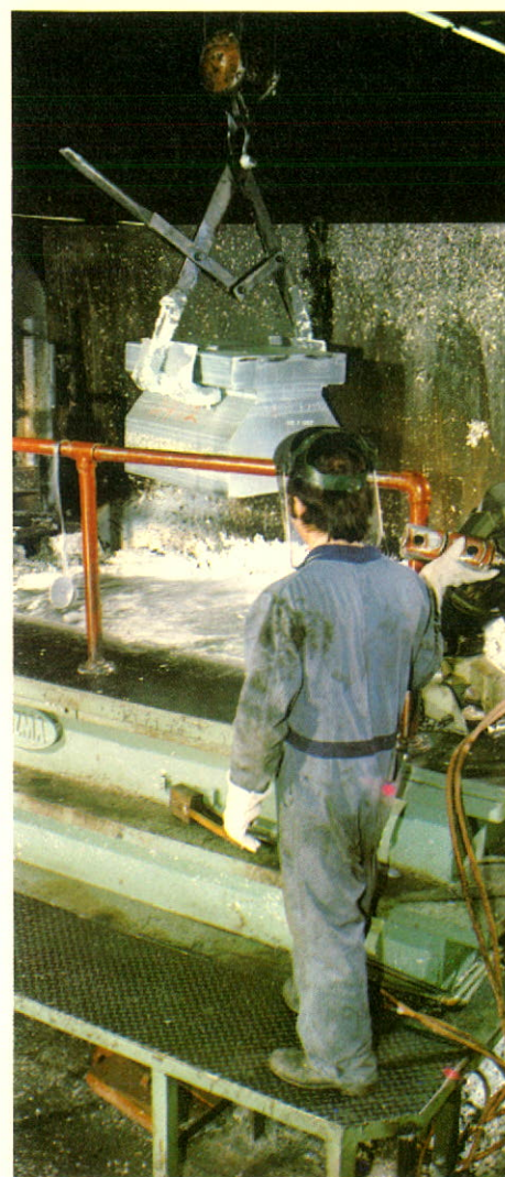
A pure zinc ingot is lowered into a furnace for primary melting and controlled mixing with premeasured alloys at Webster Mfg. (London) Limited.
