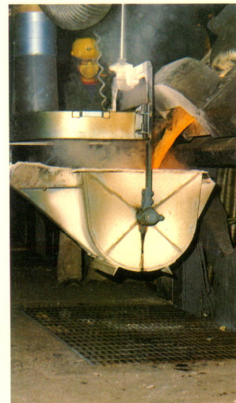
Automatic ladle for pouring bronze railway journal bearings.
