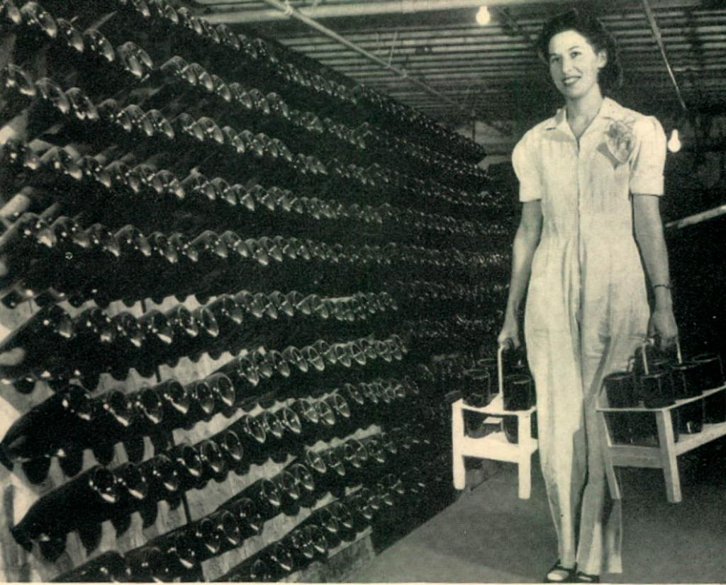
*The "pulpit"—the special racks where the champagne is held with the bottle inverted and made ready for the disgorging operation.*
