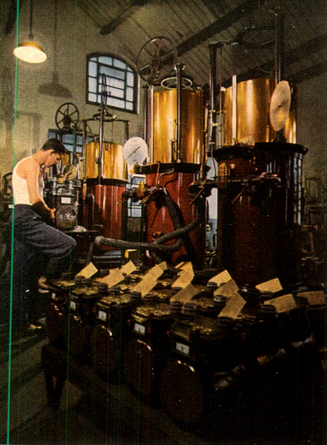
GAS METERS ARE TESTED REGULARLY.
