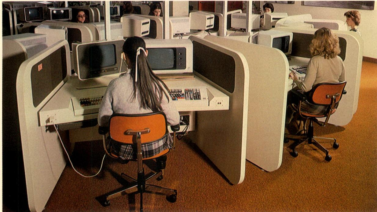
In September, NBTEL converted its directory assistance service for the southern half of the province to new, computer controlled operations. Instead of looking up numbers in paper directories, directory assistance operators use video display terminals to access numbers stored in a mini-computer. The new system is more efficient and allows faster and easier updating of number changes.
