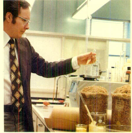
New technology for pulp and paper mills was developed in CIL's Chemicals Research Laboratories using anthraquinone in alkaline pulping. In the photo, Hutch Holton, who was responsible for the development, examines one gram of anthraquinone in dispersion, enough to produce 1000 grams of linerboard pulp. The Company considers the new technology the most important breakthrough since the introduction of kraft pulping.
