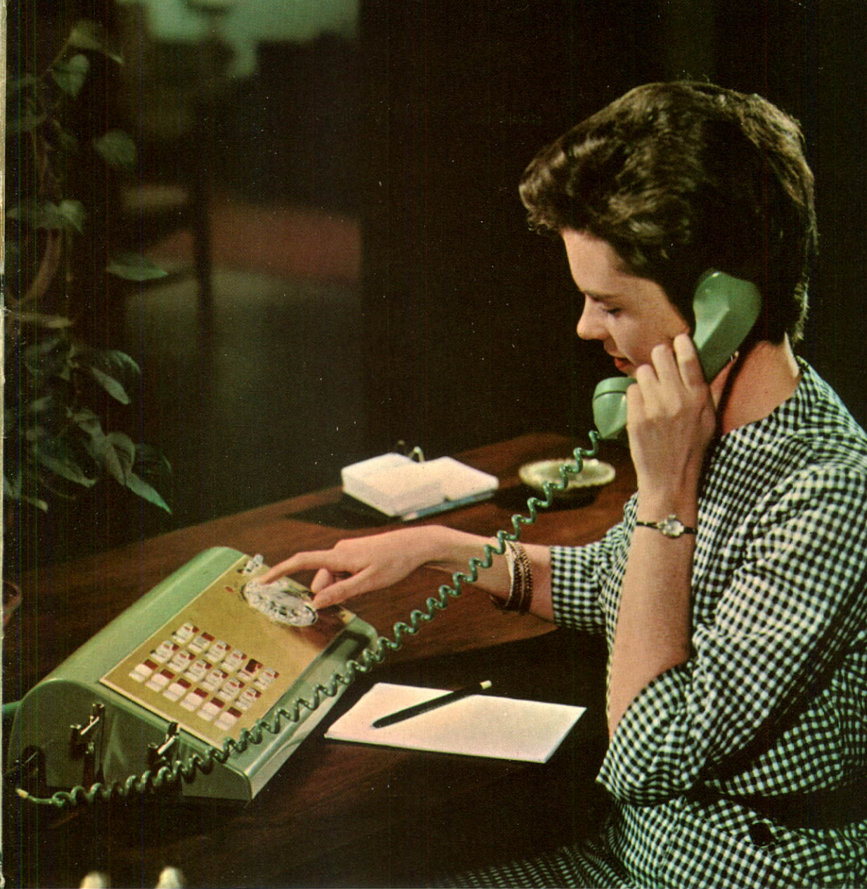
This is the desk-top control unit for our latest private exchange (PBX). Automatically, an outside call to a busy extension can be held in the equipment till the line is free, or transferred to another phone.
