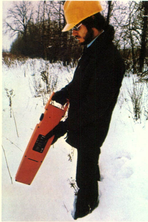
The peg locator enables telephone companies and public utilities to pinpoint underground equipment via radio frequencies.
