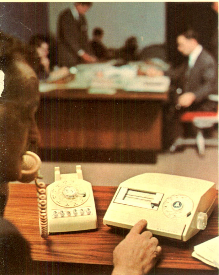
RAPIDIAL automatic dialers — first introduced in January 1962 — save precious time for this stockbroker in the Canadian Imperial Bank of Commerce Building. Telephone numbers stored in an electronic 'memory' are dialed automatically at the touch of a bar.
