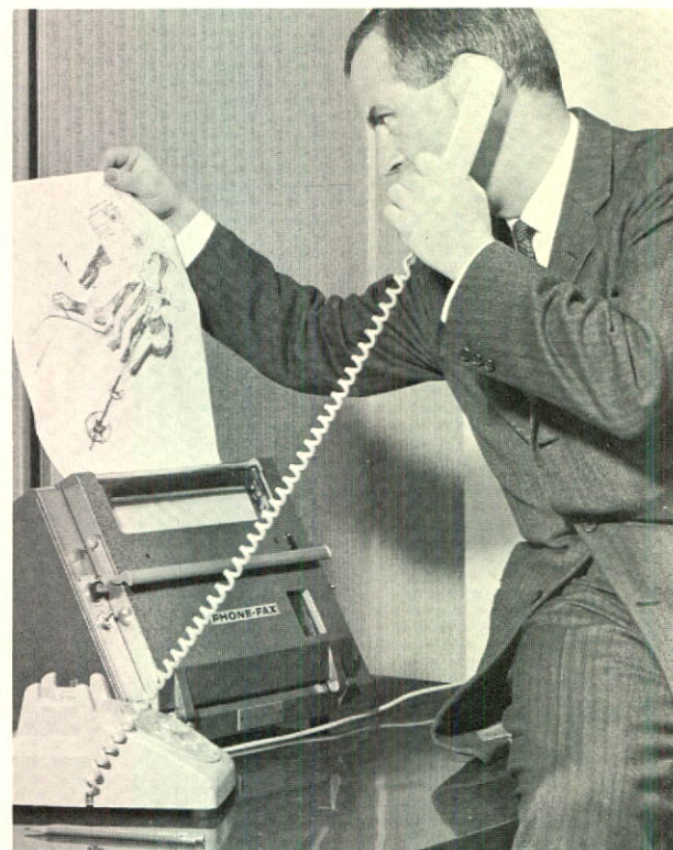
Phone-Fax service, pictured above, was introduced in March. Exact reproductions of printed material, maps and drawings are transmitted over the telephone network in a matter of minutes.
