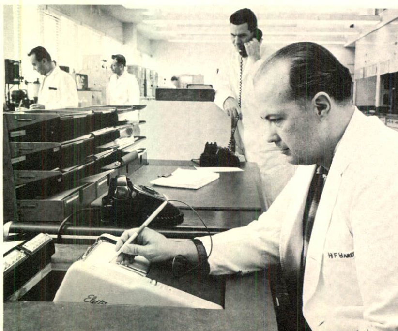
Phone-Fax service, pictured above, was introduced in March. Exact reproductions of printed material, maps and drawings are transmitted over the telephone network in a matter of minutes.
