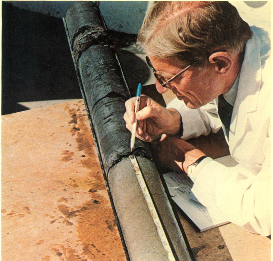
Geologist examines core from coal test well in the Pembina field in Alberta as part of program to evaluate coal seams in the area.
