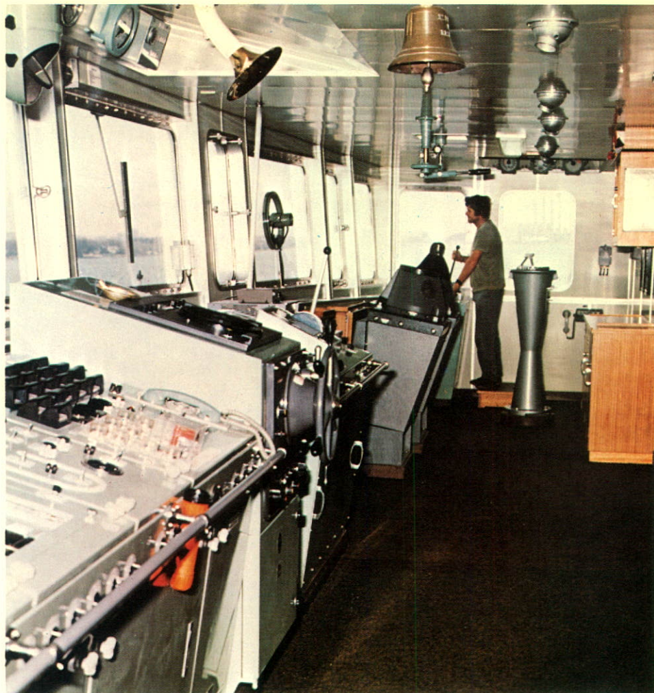
Crewman operates bow thruster control on bridge of Texaco Brave . It facilitates sensitive manoeuvring at close quarters.
