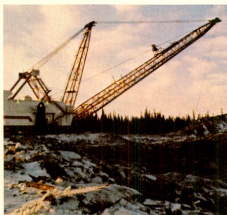
The 30 cubic yard dragline removed 7 million tons of waste and overburden in 1980.
