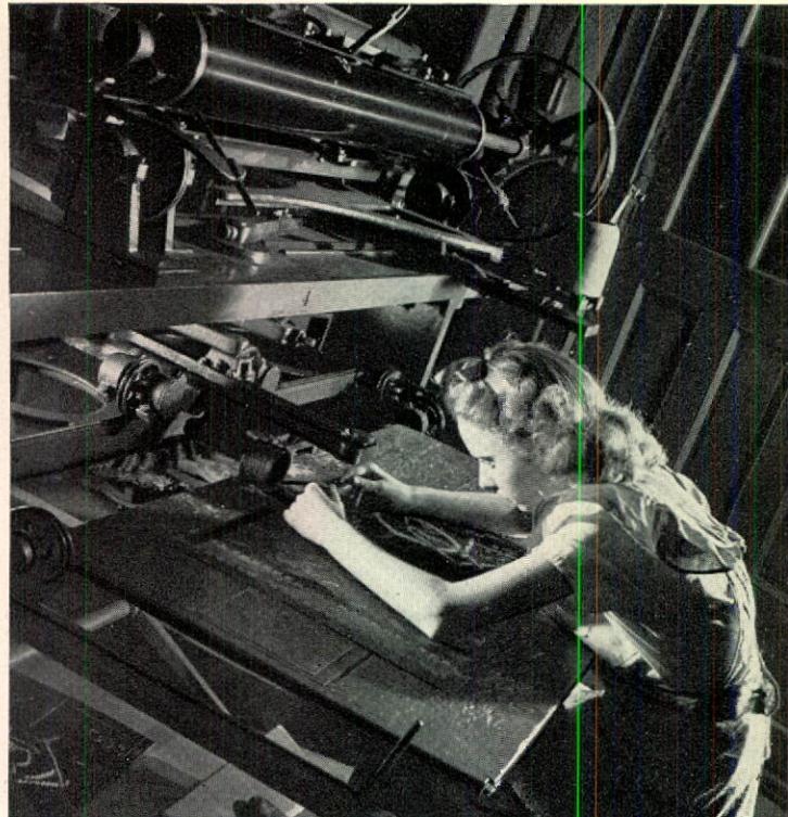
Transferring a print pattern from a flat drawing to a cylindrical copper print roller.
