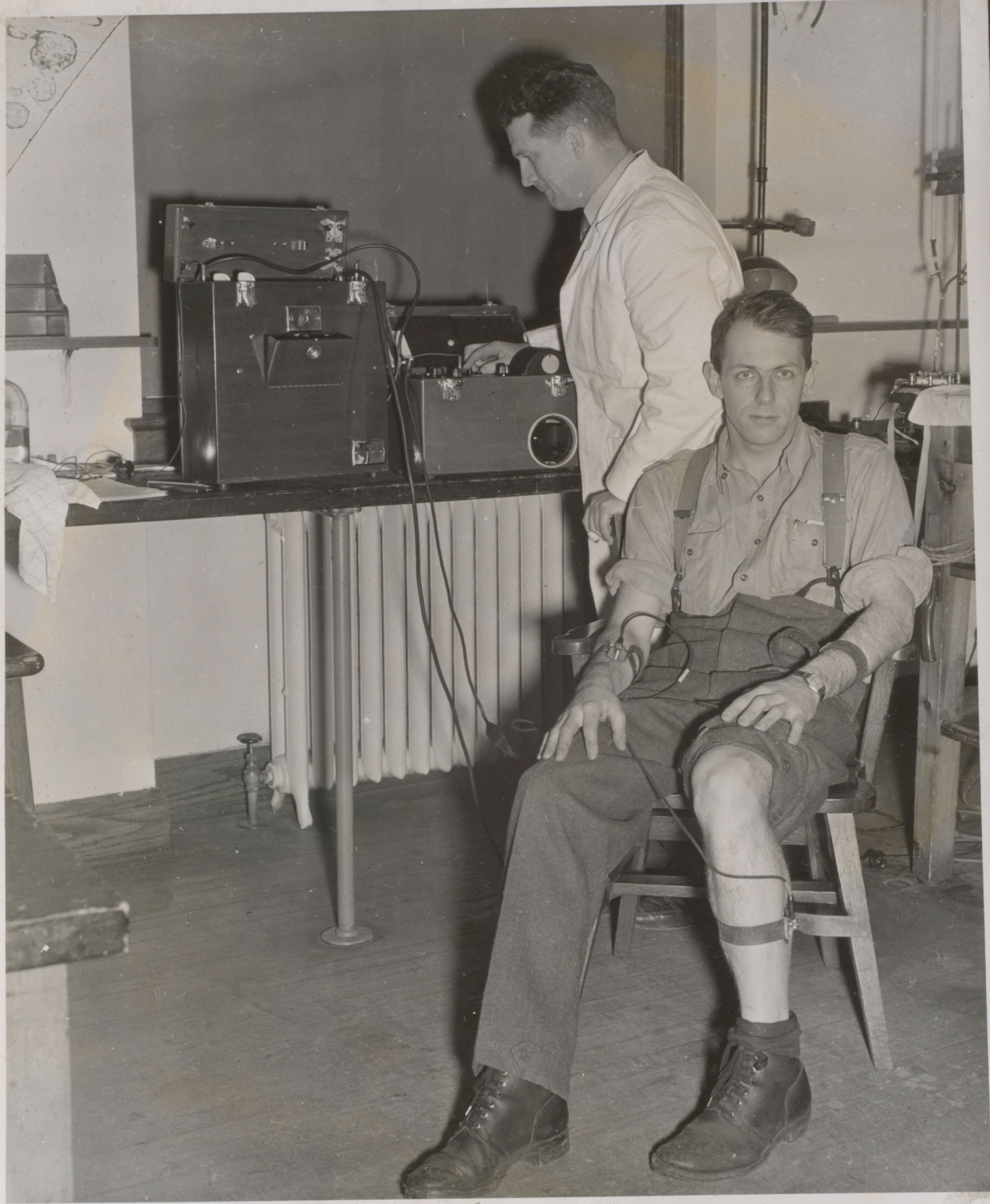
ELECTRO-CARDIOGRAPHY - DR. H.E. HOFF USING SANBORNE CARDIETTE AND CARDIOSCOPE, WHICH MAKE WRITTEN AND VISUAL RECORDS OF THE ELECTRICAL IMPULSES OF THE HEART BEAT.
