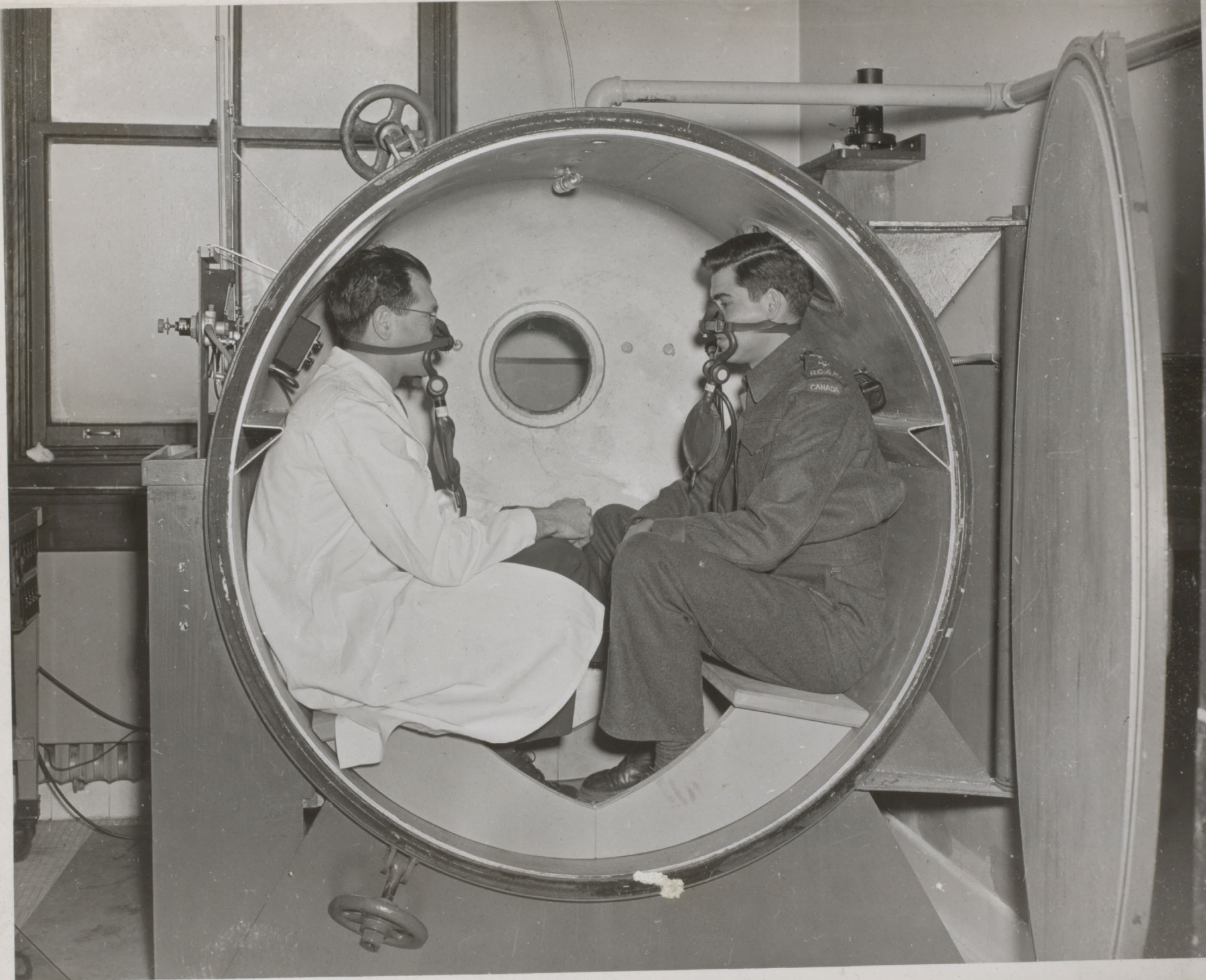
THIS SHOWS A SUBJECT, MR. MURRAY BORNSTEIN, ON THE LEFT AND AN EXPERIMENTER, CAPT. E. PETERSON, ON THE RIGHT, SEATED IN THE CHAMBER AS THEY WOULD BE DURING A DECOMPRESSION EXPERIMENT. THEY ARE SEATED ON THE REMOVABLE WOODEN SEATS. BOTH ARE WEARING B.L.B. OXYGEN MASKS. ONE OF THE ELECTRICAL BOXES IS SEEN AT THE BACK OF THE SUBJECT'S HEAD, THUS ILLUSTRATING ITS CONVENIENT LOCATION FOR TAKING ELECTROENCEPHALOGRAMS AT ALTITUDE.
