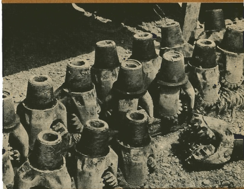
As many rock cutting bits as these may be worn out in only a few feet of hard formation
