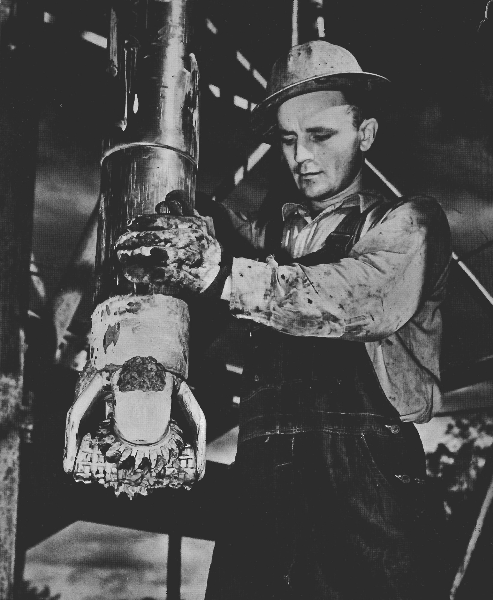
The "business" end of a rotary drill. Drilling bits such as these are used to penetrate hard formations. Sometimes the going is so hard that a bit is worn out after cutting through only two or three feet.
