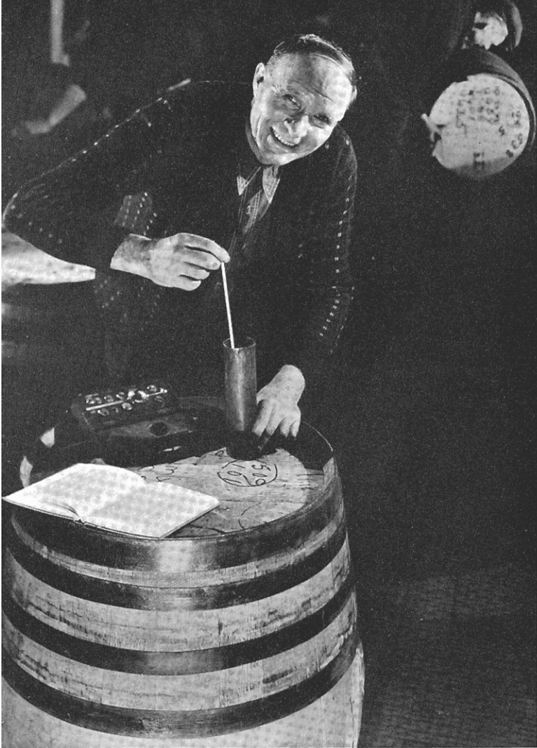
WALKERVILLE, HOME OF CANADIAN CLUB: With instruments and tables an expert tests the proof (alcoholic strength) of whiskey in storage.
