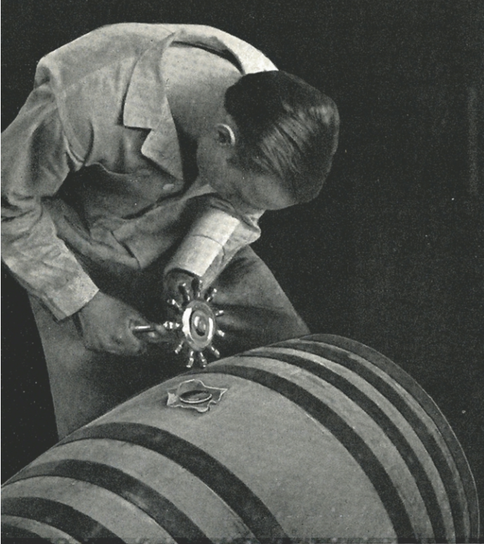
PEORIA—Visitors enjoy this detail of sealing a barrel of whiskey. The spokes of the wheel are numbered dies, which are struck into the wood of barrel and stopper to identify the contents in accordance with government records.
