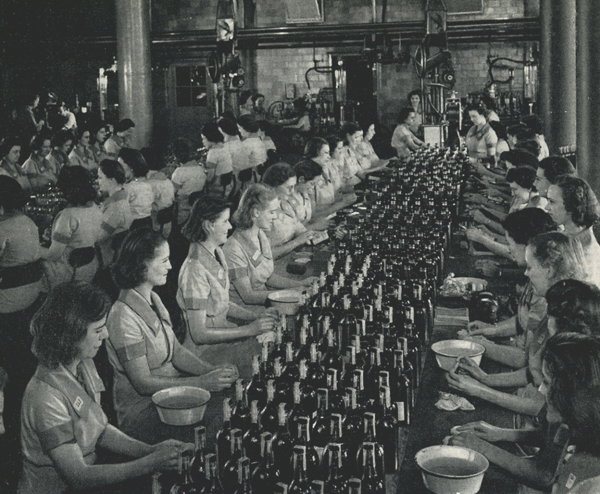
PEORIA: Hundreds of women are employed on the bottling lines, of which there are 11, with a total daily capacity of 25,000 cases. Bottles are filled, stoppered and labeled by automatic machines, but seals and tax stamps are affixed by hand.
