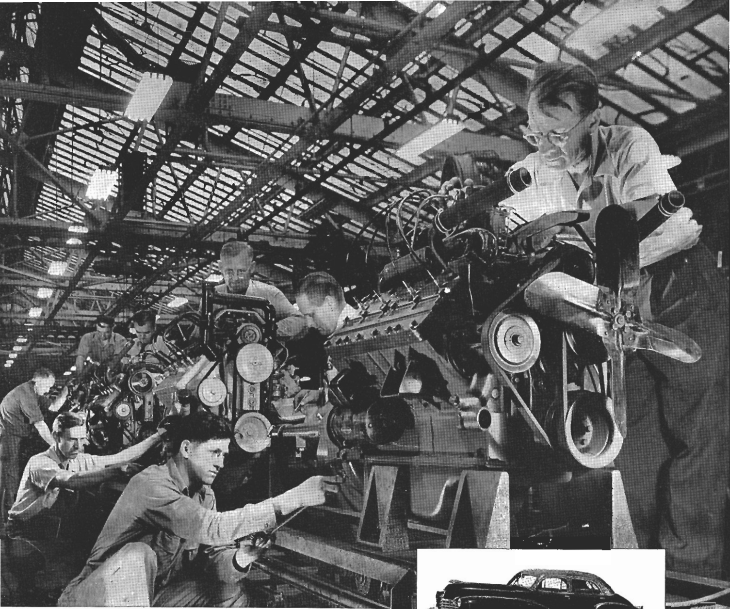
Cadillac engines on the assembly line. These engines adapted to war needs, powered Cadillac-built light tanks.
