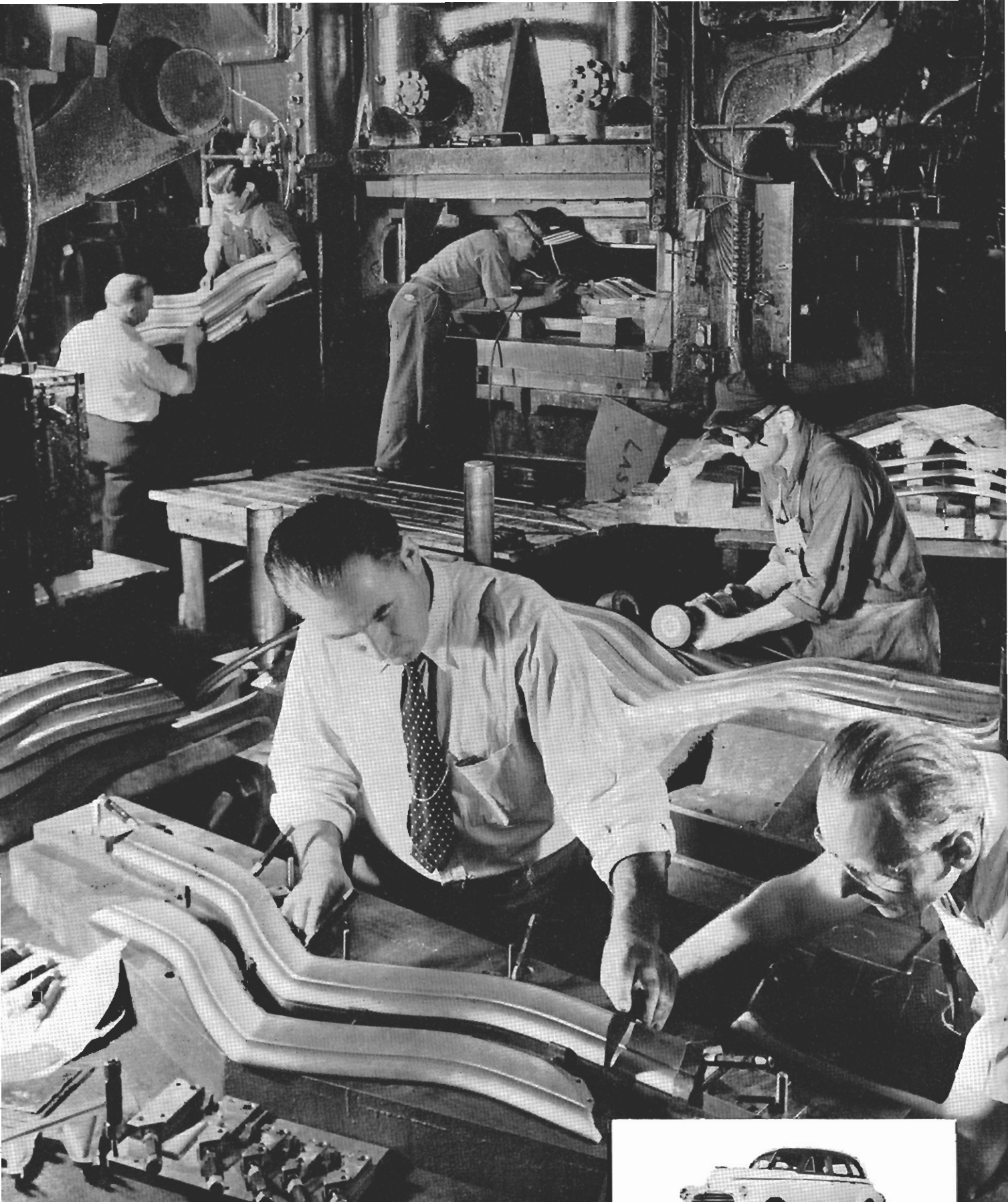
Radiator grills for 1946 Chevrolet cars are being fabricated in the scene above for the first time since automobiles became an early war production casualty. In foreground, grill parts are fitted to a jig after shaping and finishing operations are completed. Parts were stamped out on heavy press in rear.
