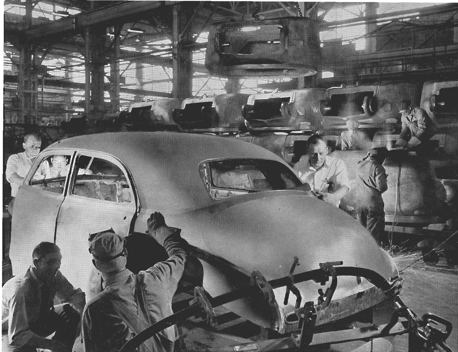
On one side of this plant welders worked on turrets to complete the final contract for heavyweight tanks for the Army. On the other side, preliminary work was being done on Fisher bodies. Pictured is a "handmade" body produced by master craftsmen in preparation for regular production.
