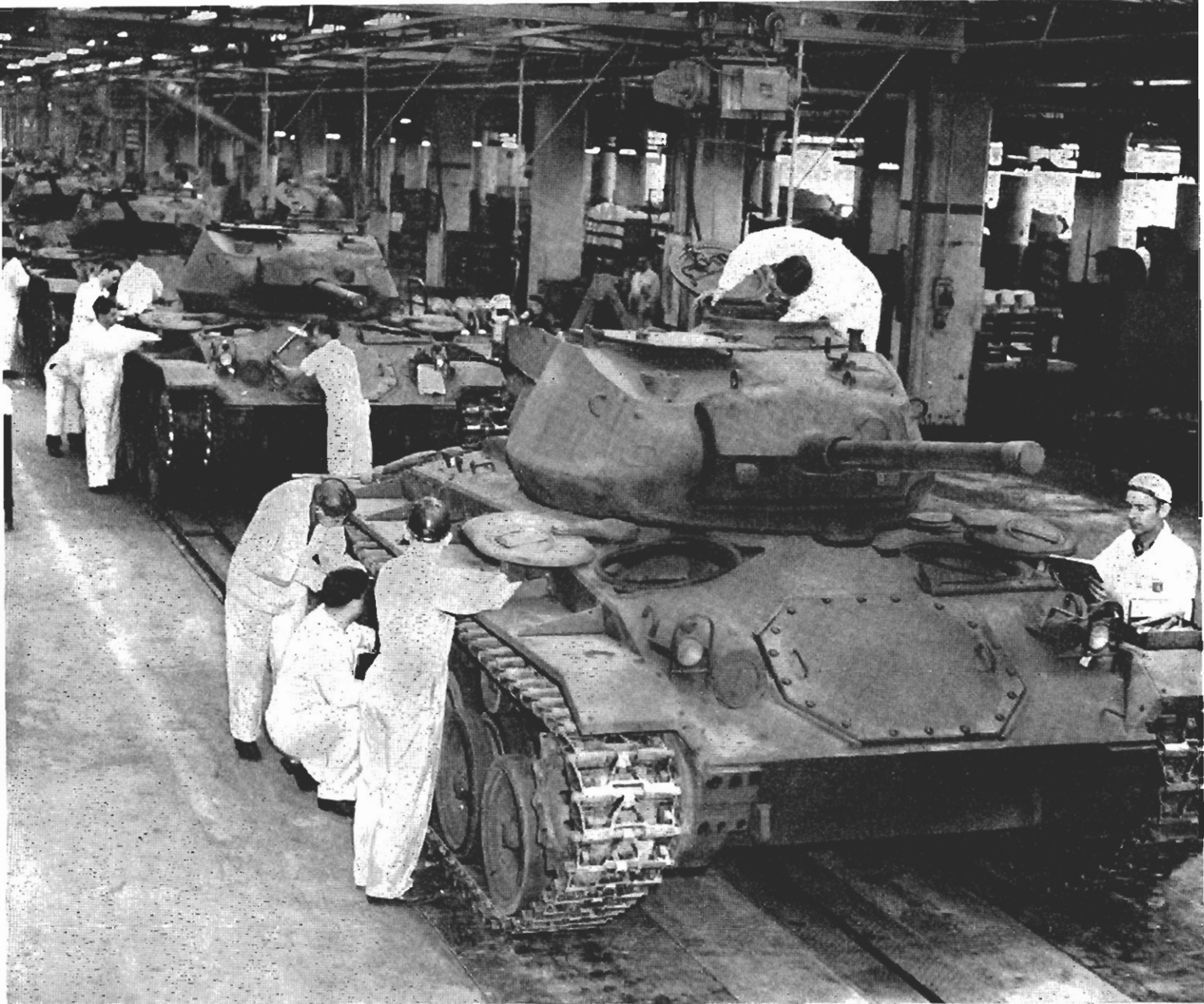
Putting the finishing touches on a line of M-24 tanks at Cadillac. The M-24, like its predecessors, the M-5 light tank and the M-8 howitzer motor carriage, is powered with two Cadillac V-8 engines driving through Hydra-Matic transmissions.
