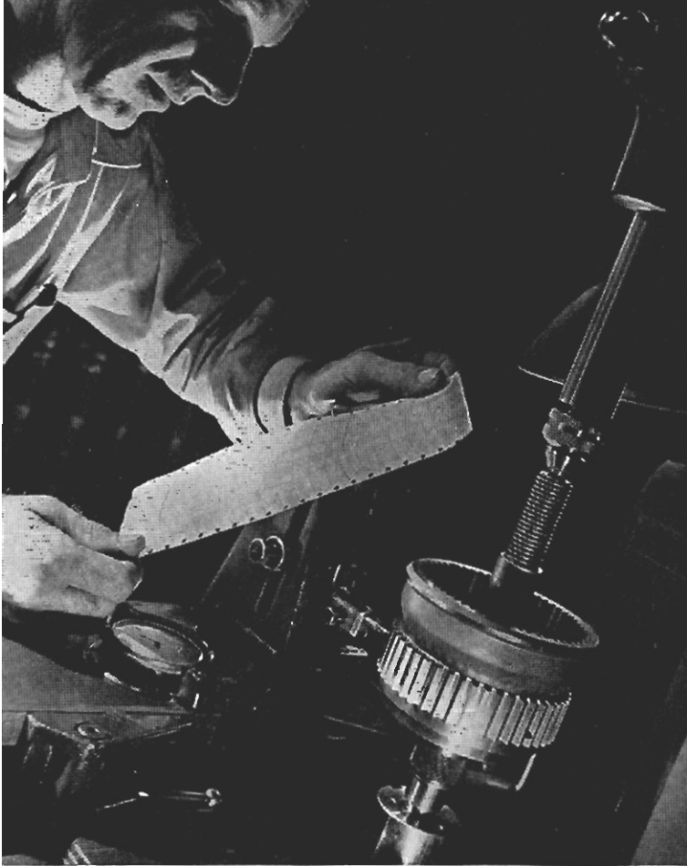
Accuracy is the first law of quality production. Inspecting a gear to one ten-thousandth of an inch tolerance at Saginaw Steering Gear Division.
