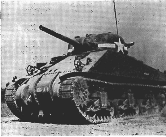
The GM-built M-4 General Sherman tank, with its all-welded steel hull, is a stalwart of the land battle fleet.
