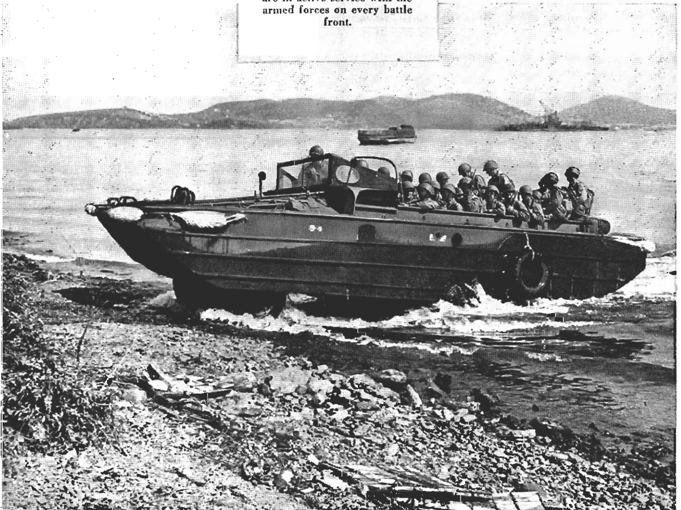
Driven by six wheels on land and a propeller in the water, the "Duck" can carry supplies or troops directly from ship to scene of battle. This GM-built invasion vehicle, shown going ashore in Italy, is one of the newest weapons in amphibious warfare.
