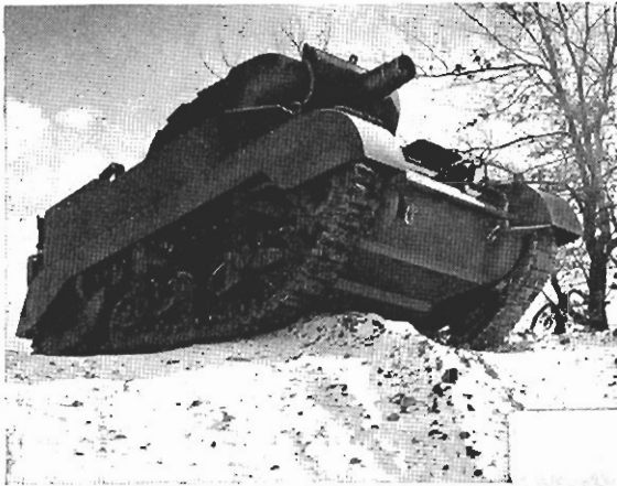
The new GM-built M-8 howitzer motor carriage uses the M-3 tank chassis and GM motive power and Hydramatic transmission.
