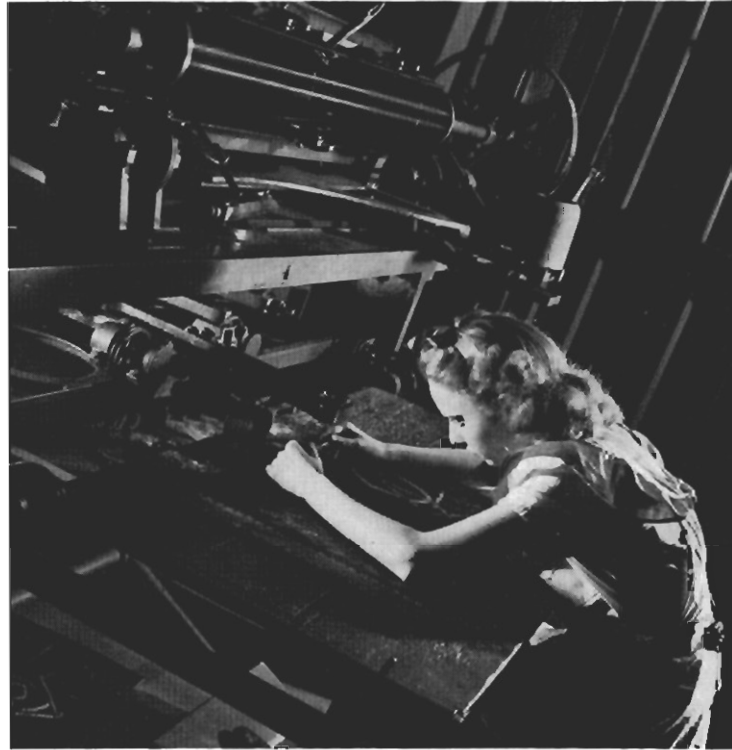
Transferring a print pattern from a flat drawing to a cylindrical copper print roller.
