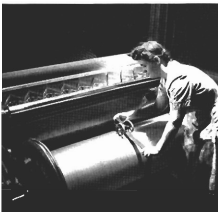
Warped threads are wound onto a large beam.
