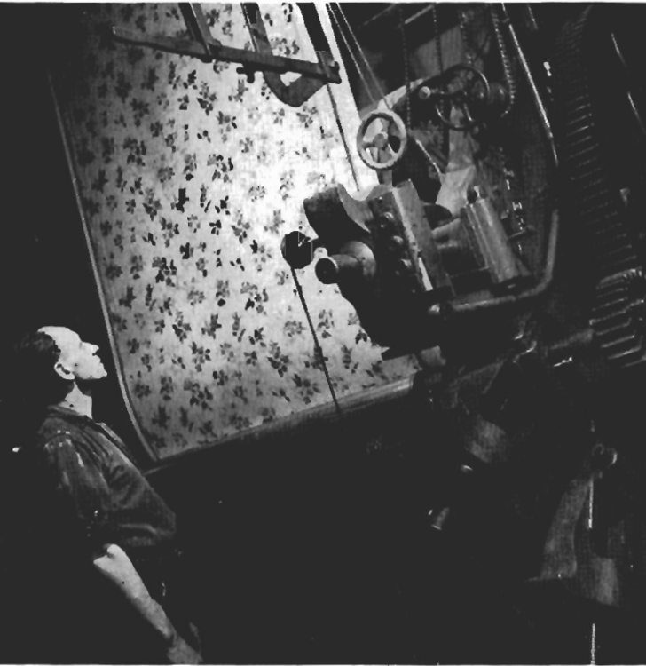
The roller printing machine applies a multi-colour pattern to a Bruck Fabric. Constant vigilance assures quality.
