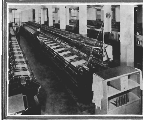
KNITTING BELDINGS AND CORTICELLI FULL FASHIONED HOSIERY IN A CONTINUOUS OPERATION FROM WELT TO TOE
