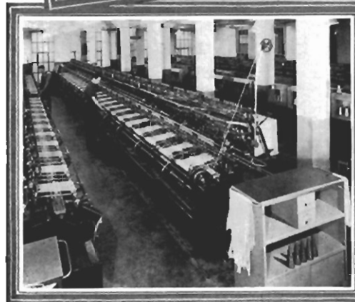
KNITTING BELDINGS AND CORTICELLI FULL FASHIONED HOSIERY IN A CONTINUOUS OPERATION FROM WELT TO TOE
