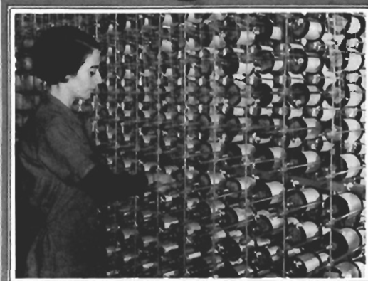
MAKING WARPS FOR BELDINGS RIBBONS ON NEW HIGH SPEED WARPERS
