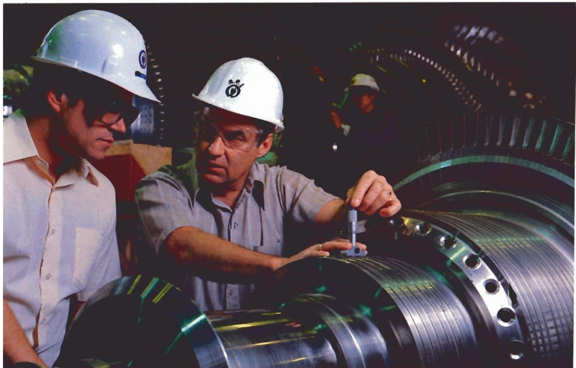
3. A. S. Brokke, right, manager of the Sheerness Generating Station project for Alberta Power, checks a rotor for the 375-megawatt turbine generator, while senior resident mechanical engineer C. H. Kerlake looks on. The first unit is scheduled to be commissioned in January, 1986.
