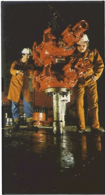
Above: Making certain it's right before it's rented, ATCO Oilfield Equipment shop mechanics inspect a blowout preventer before it is sent to a customer. Throughout western Canada, drilling and well servicing companies rely on equipment from this division. Below: right : An ATCO Well Servicing rig at work in southern Alberta. Similar equipment is located throughout western Canada and the U.S. and one rig now is operating in Australia, enhancing recovery from existing wells and completing new ones.
