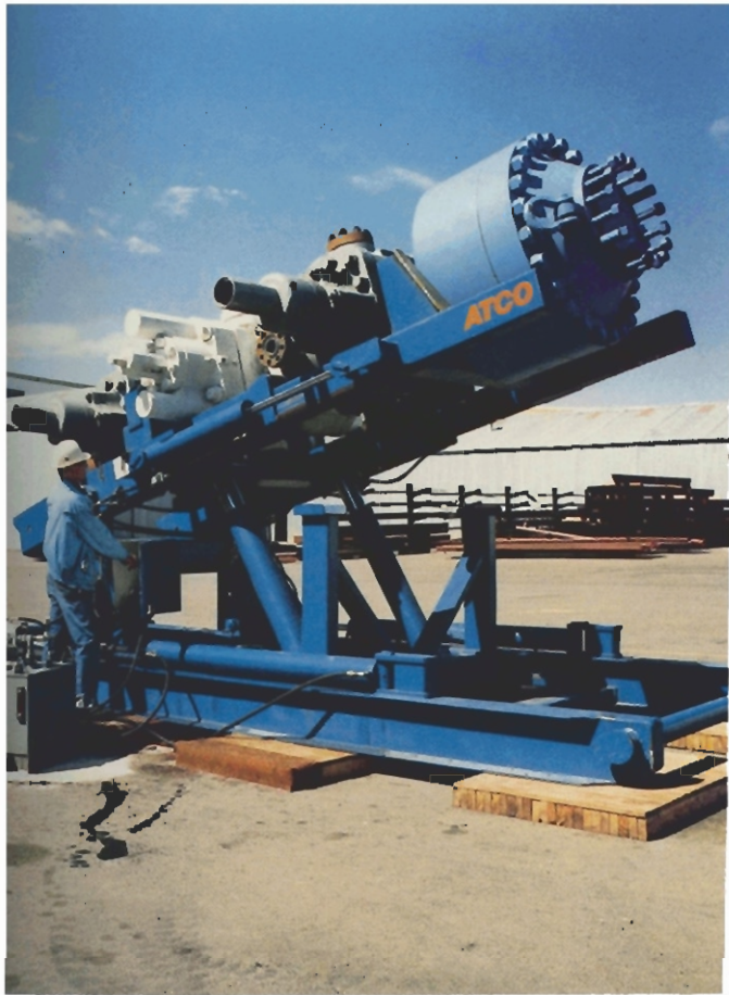
Blowout preventer cradle designed and manufactured by ATCO Metal Ltd.
