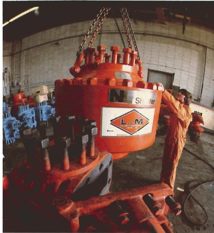
L & M sells and rents specialty oilfield equipment such as this blowout preventer.
