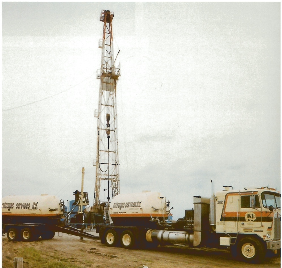
Opposite page top: Acid unit servicing a well in Central Alberta
