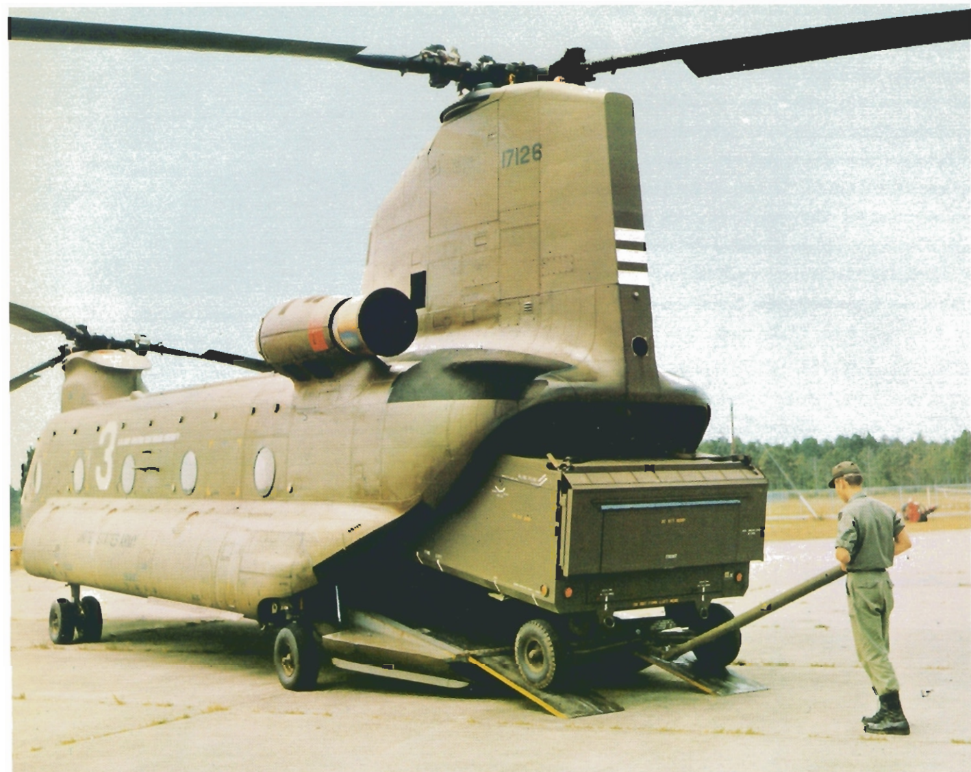
Air transportable maintenance shelters developed by the R & D Center undergoing U.S. Army testing procedures at Fort Rucker, Alabama.
