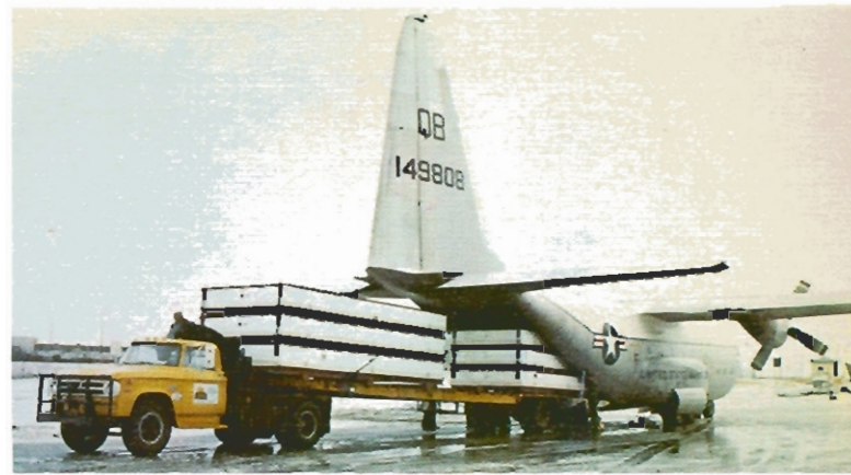
Sems modules in knock-down configuration are air lifted to the destination.
