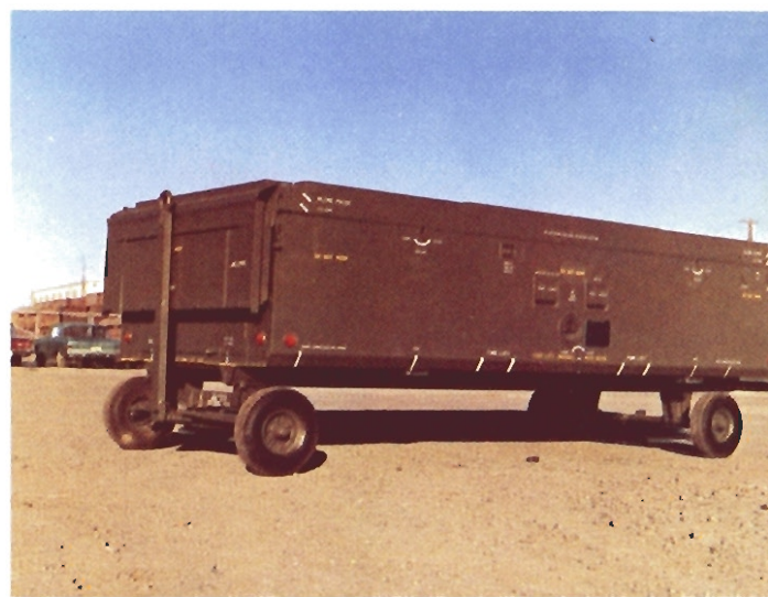
The R and D Center's Airmobile Maintenance Shop (A.M.S.) offers a vertical expansion of 2:1. The building is constructed of a unique honeycomb, sandwich panel material developed by the company.
