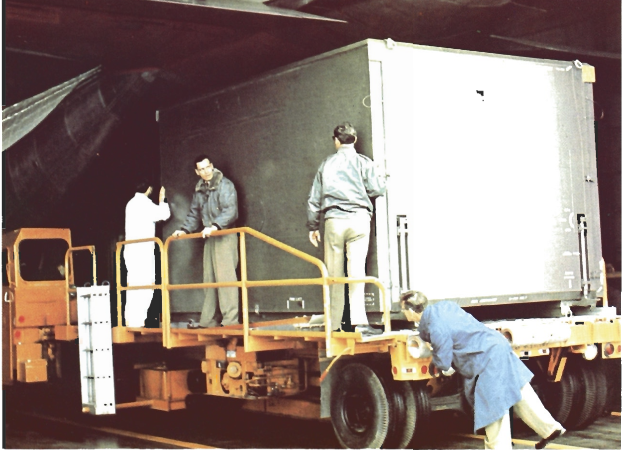
Technicians supervise test loading of an ATCO Multipurpose Expandable Shelter into hold of a Hercules aircraft. This building expands laterally to a volume three times its shipping size.
