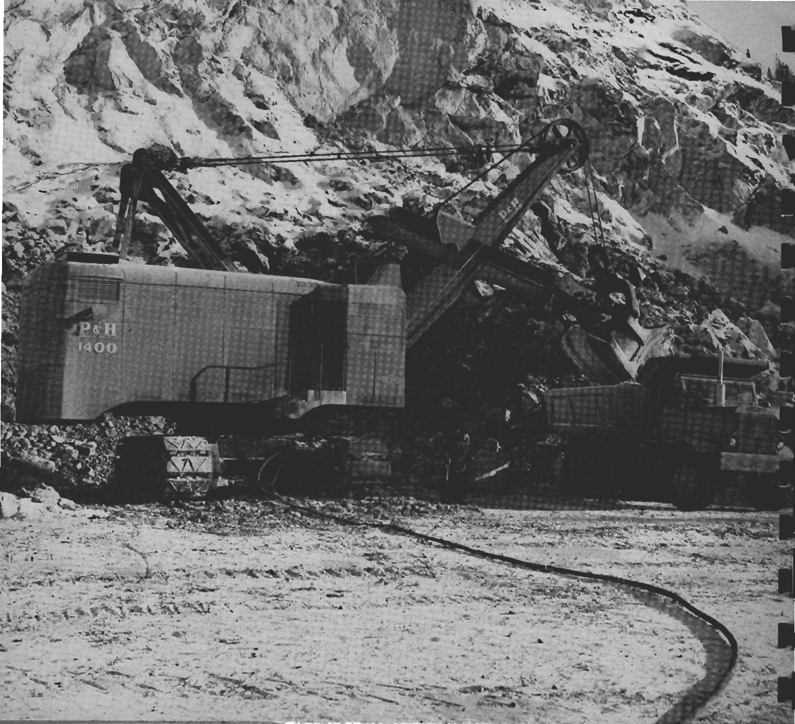
4 Cubic Yard Electric Shovel Loading Diesel Truck at Pit Face British Canadian Mine.
