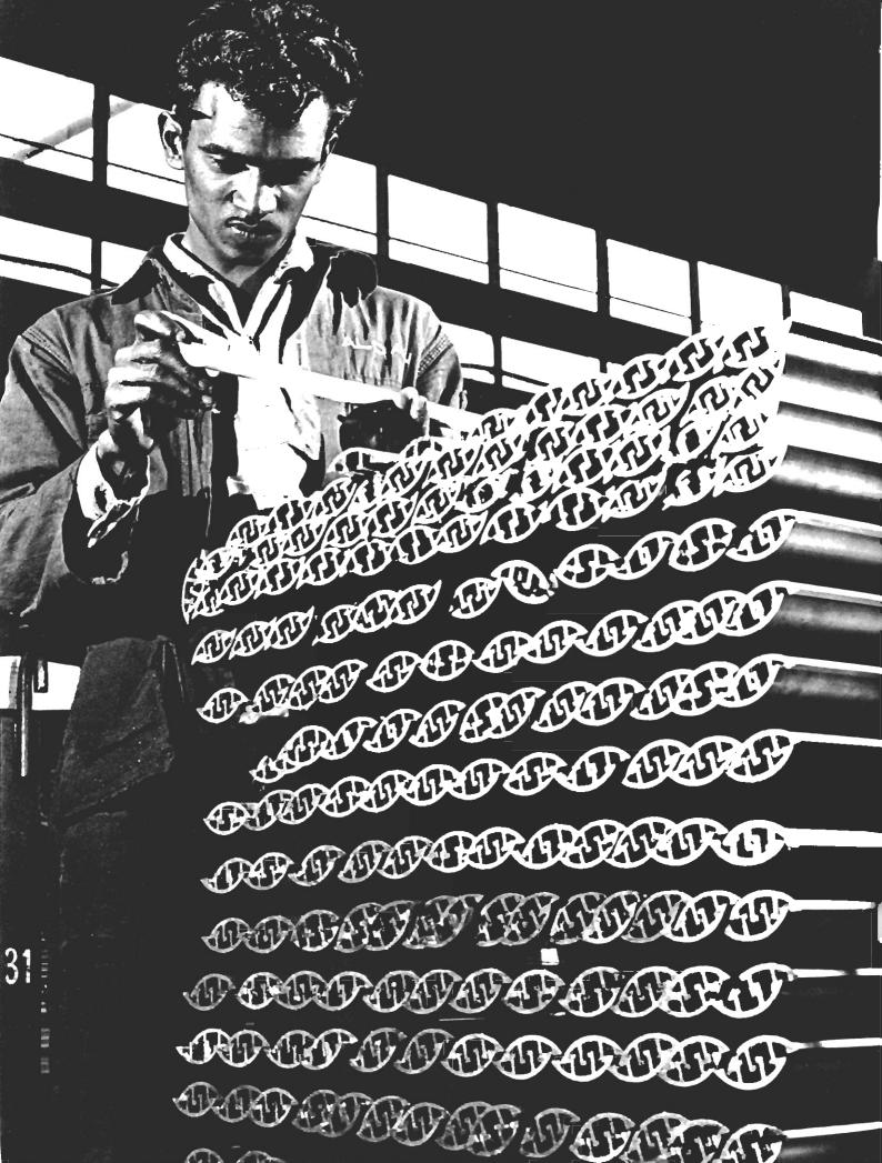
Aluminum is particularly well adapted to the extrusion method of fabricating, producing shapes and profiles of intricacy and strength without loss of economy. This employee of Alcan Aluminium of South Africa contributes his essential skill to the success of the operation.
