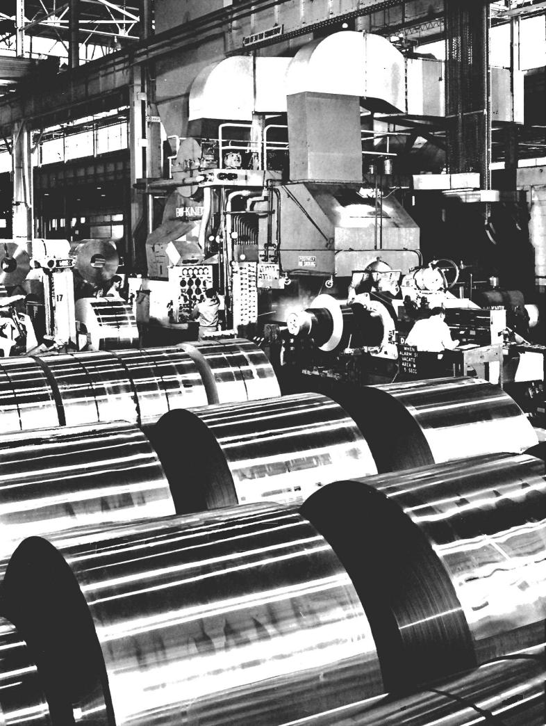
Modern cold rolling facilities of Alcan Aluminum Corporation at Warren, Ohio, and coils of aluminum sheet ready for sale to manufacturing customers.
