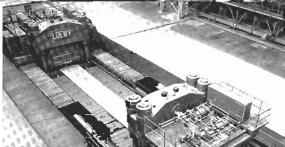
The continuous strip mill at Rogerstone showing the 700 ft. long runout table and hot finishing mill
