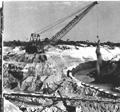
Removing overburden at Montgomery mine in British Guiana. This walking dragline has a 220 foot long aluminum boom, scoops 13 tons each time
