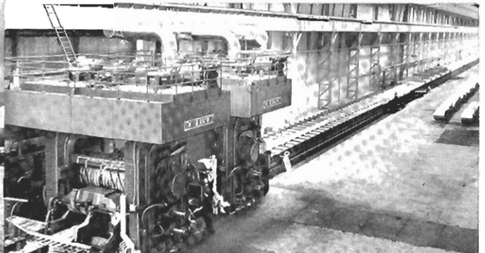
The continuous strip mill at Rogerstone showing the 700 ft. long runout table and hot finishing mill
