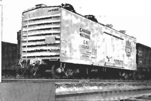
Aluminum refrigerator car developed by Alcan, C.N.R. and National Steel Car. Rolling stock is major new aluminum outlet
