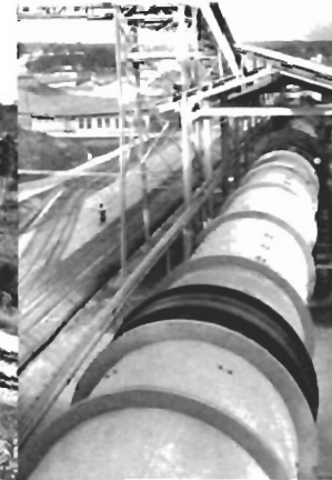
Giant kilns at the Mackenzie, B.G. ore plant dry the bauxite. Three kilns also calcine the ore for the abrasive and refractory industry
