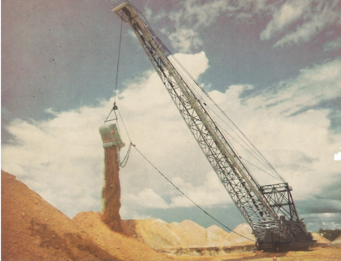
the world's largest working dragline using an aluminum bucket scoops up 30 tons of British Isotona bauxite
