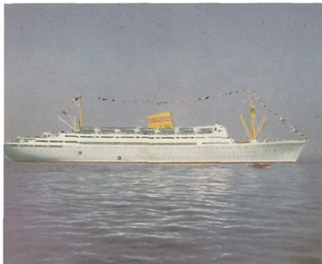
The S.S. Bergensjord incorporates the largest marine use of all-welded aluminum structures.
