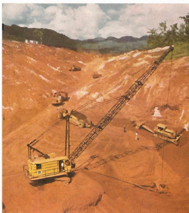
Open pit mining of Jamaican bauxite for the adjacent alumina plant at Kirkvine Works.
