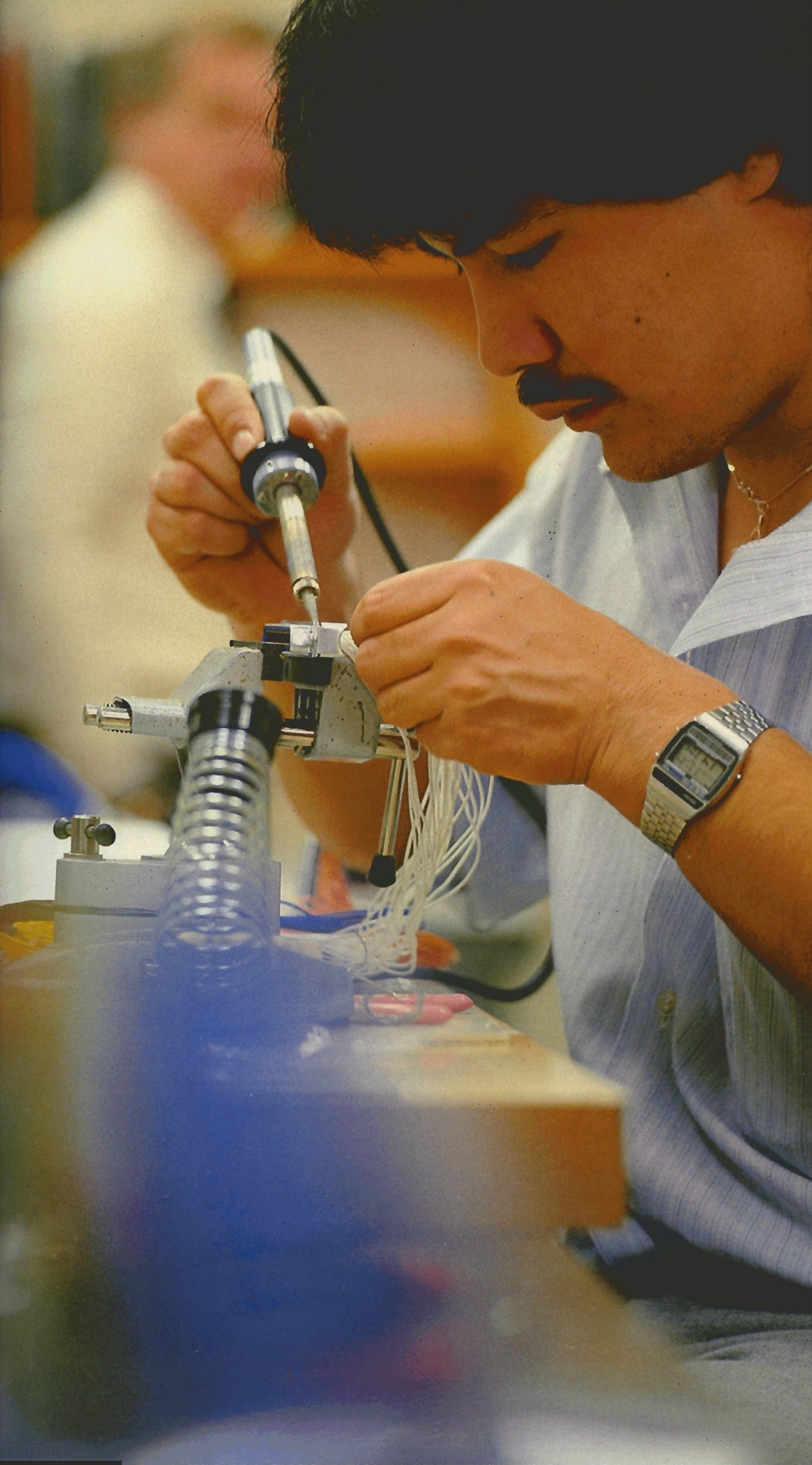
Dave Adachi, an inspector at Amphenol Products, prepares a fixture for computer testing of the 57 SERIES filter connectors used in the telecommunications industry (left). Amphenol's commercial filter connector products are widely used in computer and telecommunications installations (above).
