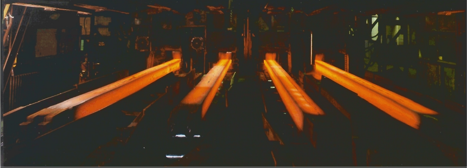
Continuous casting of blooms for rail, tubular and structural products.
